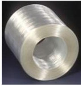
ECR-10K spray up roving is made of standard ECR-glass multi-end fiberglass
