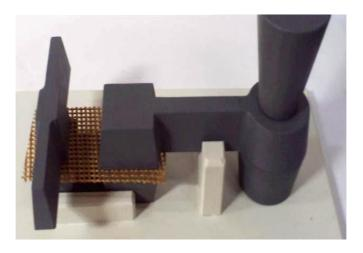
The mesh filter is better placed in the mold cavity or castings as close as possible. In this way it will reduce breakages and capture more sand slag.
