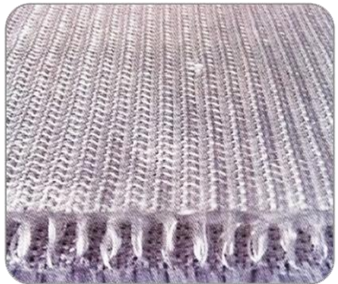
Above: Woven structure of 3-D Sandwich
