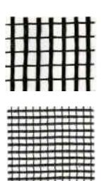
Used on new and old major roads, the material is paved between the base course and the top course, or between the top courses. It can effectively improve surface stress distribution, resist and retard the surface cracks arising from the base course cracks, and therefore the highway road service life is prolonged - and its construction cost is lowered compared to that of traditional roads and pavements.
